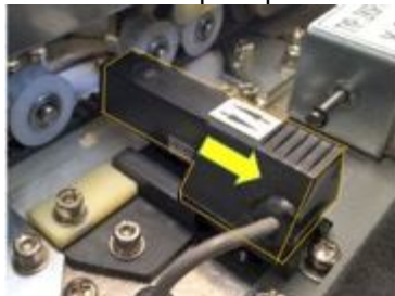
Coin sensor "Open" position
